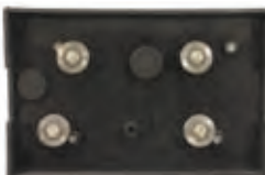
RW-XL Thread Carriage Has 4 metal rollers
