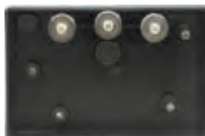
RW-3XL & 3L Thread Carriage Has 3 metal rollers
